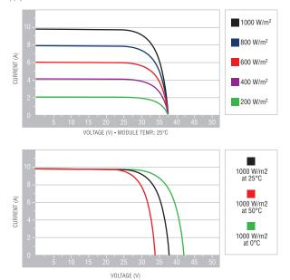
\*STC: (Standard Test Condition) Irradiance 1000W/m²; Module Temperature 25°C; Air Mass 1.5
