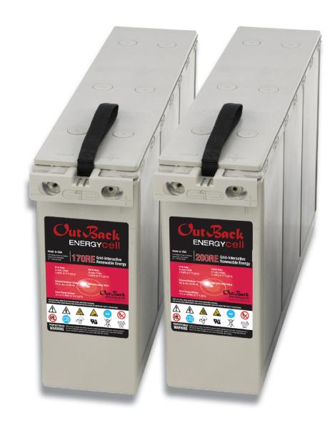
The EnergyCell RE Valve Regulated Lead Acid (VRLA) battery is designed for high power density and renewable energy cycling applications. Absorbed Glass Matt (AGM) technology provides for efficient gas recombination of up to 99% and freedom from electrolyte maintenance. The EnergyCell RE also features low profile terminals with threaded copper alloy inserts providing reduced maintenance and increased safety.
