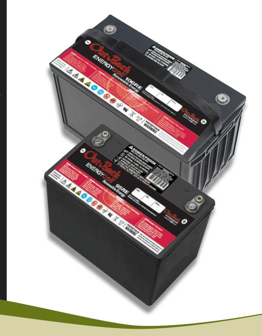
The EnergyCell RE Top Terminal valve regulated lead acid battery is designed for high power density and renewable energy cycling applications. Absorbent Glass Mat (AGM) technology for efficient gas recombination of up to 99% and freedoom of electrolyte maintenance. The EnergyCell RE also features low profile terminals with threaded copper alloy inserts providing increased safety and reduced maintenance.
