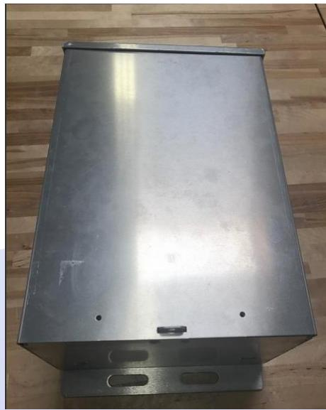
The BBA-Mini is the smallest aluminum enclosure that we carry. Pole or wall mountable (mounting hardware not included), the BBA-Mini can hold a single Group 22NF lead acid battery. The 9.75" x 4" backplate can fit a smaller charge controller along with breakers and terminal blocks. Two knockouts on the back and two on the bottom give installation flexibility. The screw cover is lockable as well.
