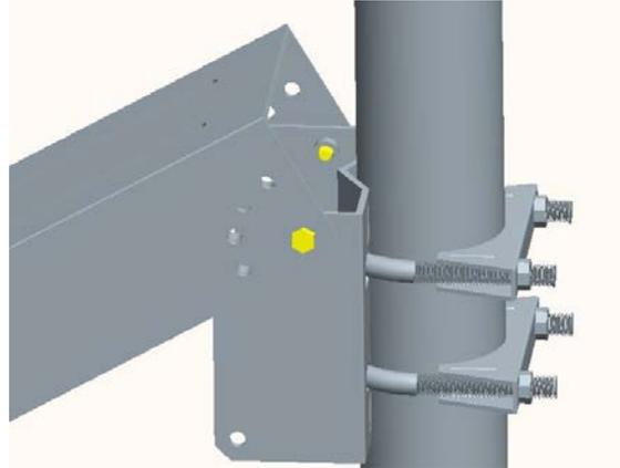
Adjust the arm piece to desire angle and insert the bolt from outside and insert the washer from inside and tighten the bolt. Make sure you have two sets on each side installed.
