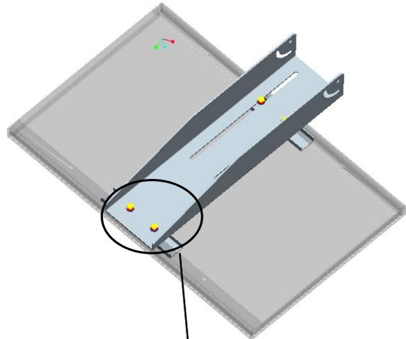
Make sure that the clamp bolts are resting against the module's flange before tightening
