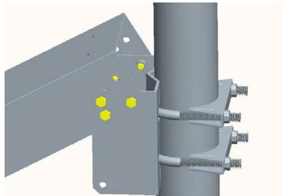
Adjust the tilt of the panel as desired, and tighten the bolts
